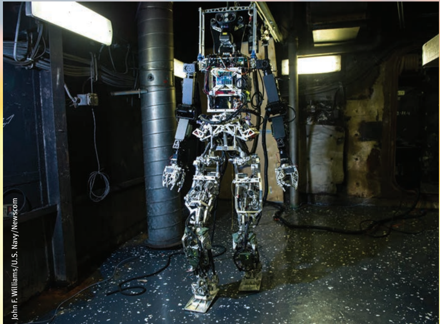
The Shipboard Autonomous Firefighting robot undergoes testing aboard the Naval Research Laboratory's ex-USS Shadwell in Mobile, Alabama.
