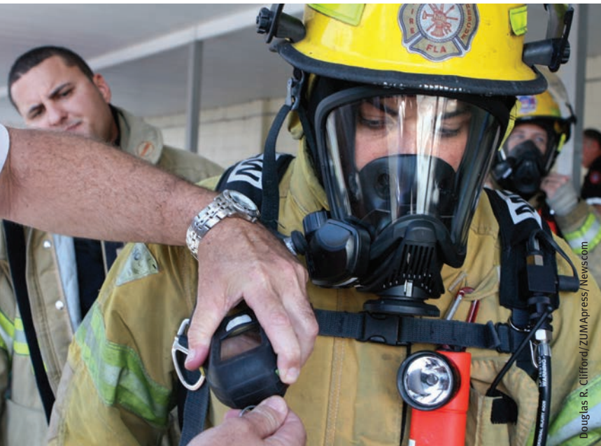
Above left: Before a training exercise using a new self-contained breathing apparatus, a training chief synchronizes a firefighter's incident control module with the district chief's computer—allowing remote monitoring of temperatures inside structures and heart and oxygen rates of firefighters, in addition to remote signaling used to recall firefighters. Above right: Through the Congressional Fire Training program, Congressional staffers are put through exercises that firemen in training would encounter, including use of a thermal imaging device.
