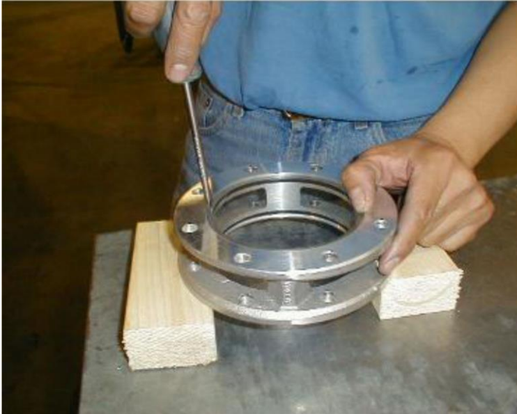
Figure 1 – Sight Glass Removal
