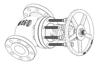
Lift the bonnet and stem assembly out from the body. Remove the gasket.
