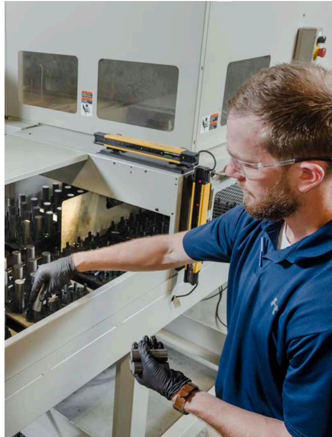
Left to Right: In process quality. A work center operator inspecting a fresh crimp prior to machining; Plasma Cutting of metal sheet stock -- the first step in producing crimp sleeves or ferrules; Gantry-style robotic machining centers equipped with simple and safe loading buffers. This allows one operator to tend multiple machines.
