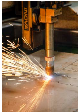
Left to Right: In process quality. A work center operator inspecting a fresh crimp prior to machining; Plasma Cutting of metal sheet stock -- the first step in producing crimp sleeves or ferrules; Gantry-style robotic machining centers equipped with simple and safe loading buffers. This allows one operator to tend multiple machines.
