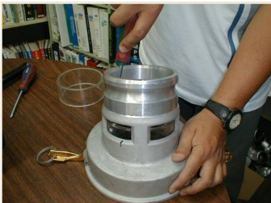
Figure 4 – Sight glass removal
