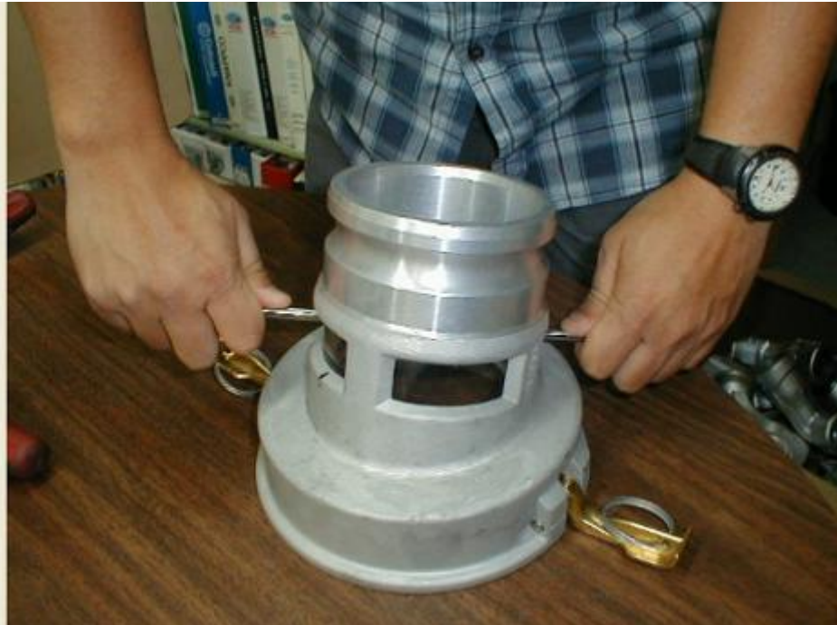
Figure 3 – Sight glass removal
